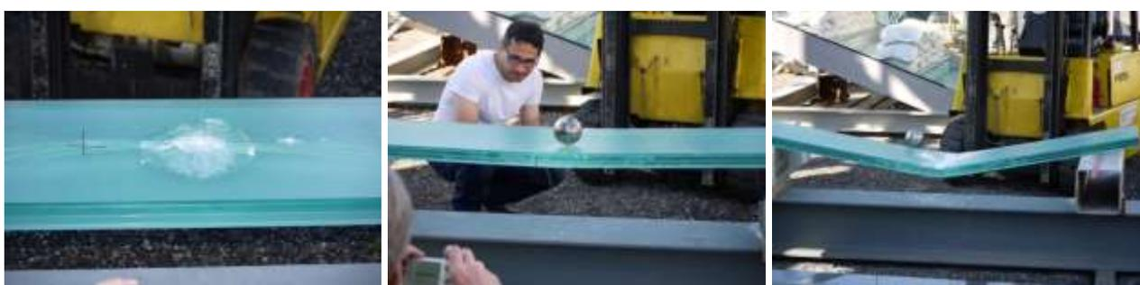
Figure 6. Some photos of hard body impact test for “Step 8.15.15.8” specimens.
