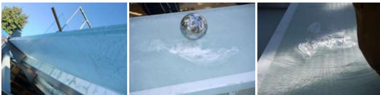
Figure 5. Some photos of hard body impact test for “Step 8hs.12hs.12hs.8hs” specimens.
