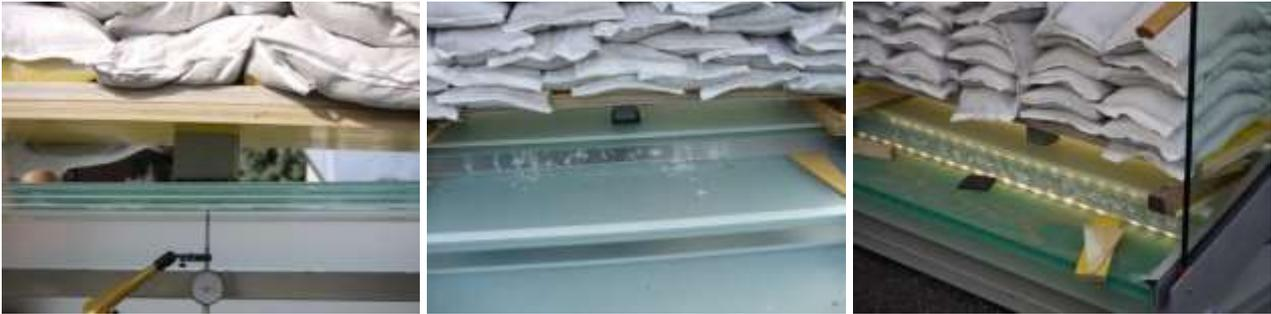
Figure 3. Concentrated load test for “Step 8hs.12hs.12hs.8hs № 1, 2 and 3” specimens.
