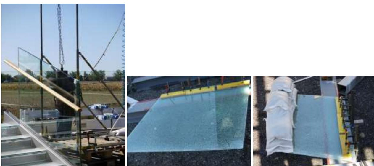
Figure 7. Tests of “Barrier 12t.12t” specimens for soft body impact and linear distributed load.
