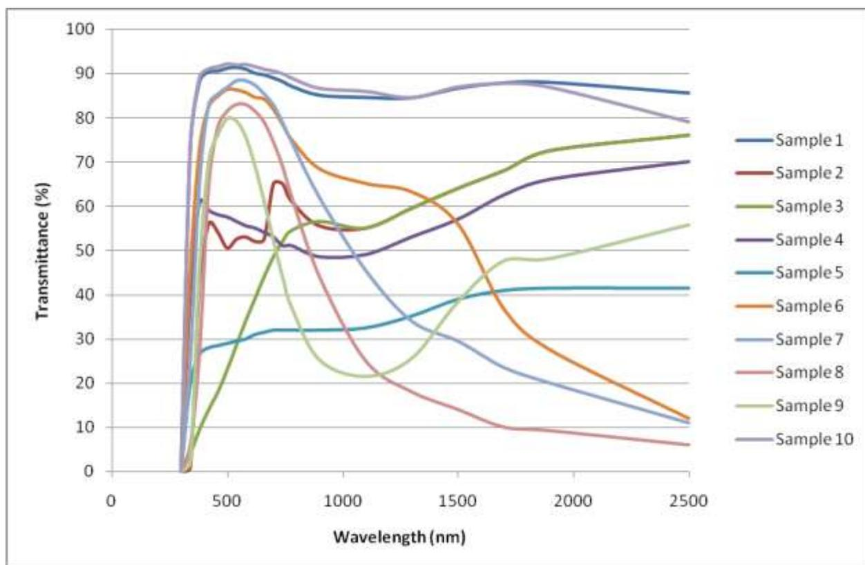
Figure 2 Transmission spectra characters of the analyzed glass specimens
